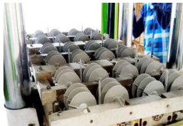
Part Name: 11 kV Composite Insulator Number of Cavities: 24
